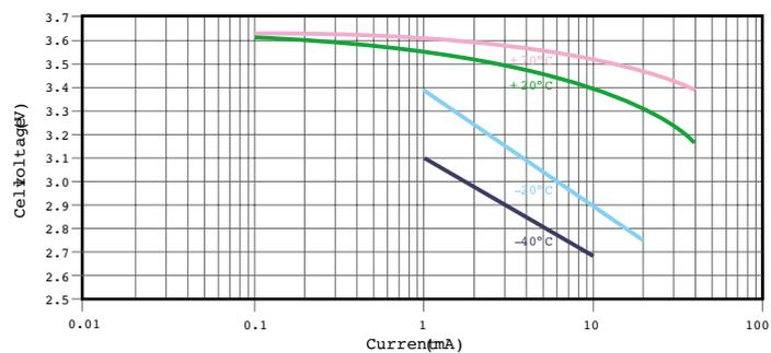
Typical discharge profiles at +20°C
